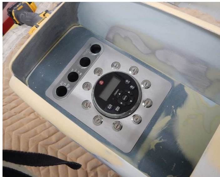
The console houses operational buttons, a Clarion radio head, and Vintage Air controls.
