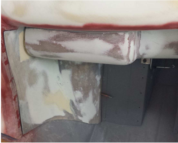
Panels made by John to encapsulate the lower dash.
