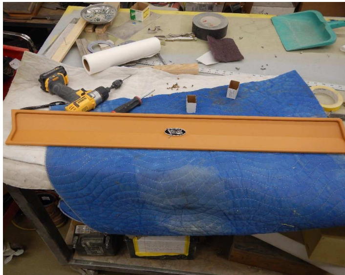
Our sill plates are made of aluminum, painted body color with a leather inset.
